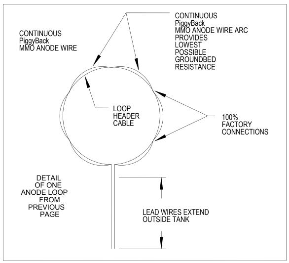
DETAIL OF THE PiggyBack Anode™ LOOP ASSEMBLY
